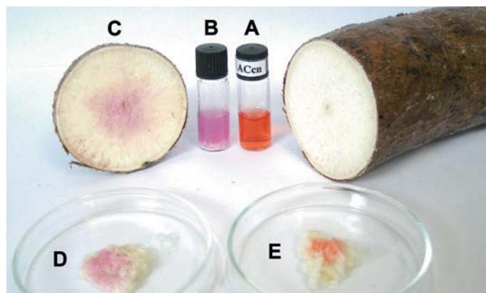
The orange corrin-based chemosensor (A) turns violet in the presence of cyanide, as in an aqueous solution of crude cassava (B), a freshly sliced cassava surface (C) or a ground cassava extract (D). No cyanide is detected after thorough washing of the ground cassava extract (E).
