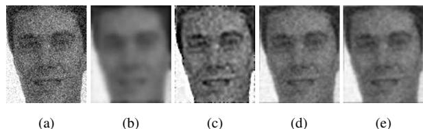
Figure 12: Respectively Noise face image with  $\sigma = 0.01$  (a), denoising without (b) and with (c) strength classification for the first method, denoising without (d) and with (e) strength classification for the second method.
