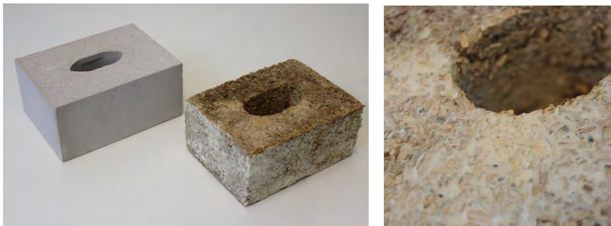
Figure 2: Mycelium-based brick prototype with sand-lime brick model (left) and close-up of the surface (right)
