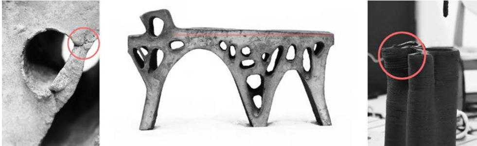
Figure 8. Flaws in fabrication. From the left: cracks, deformation of concrete casting and displacement in printing.
