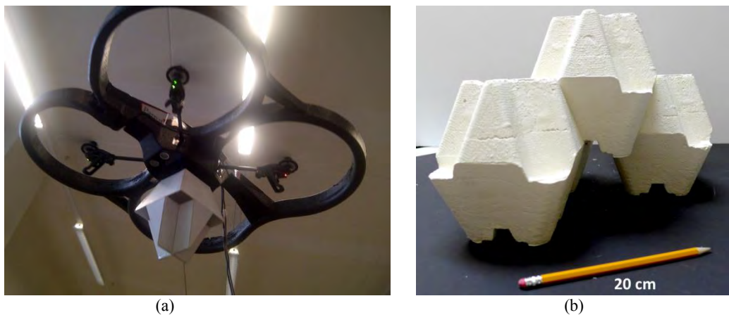
Figure 9: (a) A rigid paper droxel, lifted by the drone with a magnet during the tests; (b) Full-scale droxels cast in plaster in CNC-milled foam moulds
